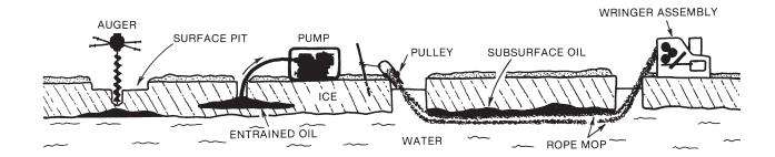
A sump is cut in the ice around a hole augered through the ice to pockets of oil under the ice or encapsulated in the ice. The oil is pumped directly from the sump to temporary storage containers. A heated shelter can be erected over the sump
