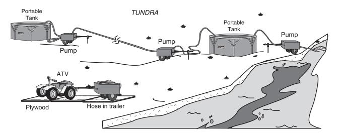
A system of hoses and pumps in series system is assembled to transfer stored liquids. Four- or 6-inch discharge hose is used in sections, with 4-inch or 6-inch trash pumps in series approximately 1,000 feet apart. Liquids are pumped to a storage tank or vacuum trucks, or are recycled into a pipeline. Hose and pumps in series are typically used across tundra, but if the hose crosses a road or pad, crossings are flagged and constructed with timbers over the hose. The hose is clearly marked.
