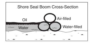
Shore Seal boom is bottom-founded and anchored at tideline and in very shallow water. Sorbent boom would be used at connections to prevent leaching.
