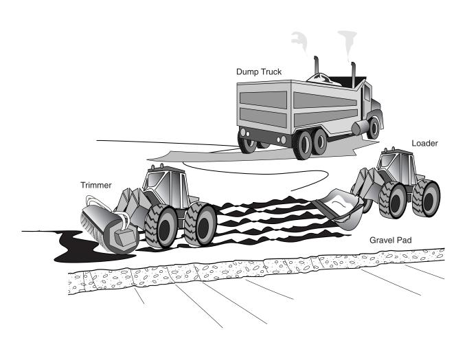
A trimmer is used to recover oil embedded in the surface of a frozen pad or ice. A trimmer uses a rotary blade system to chop and collect the surface material at varying depths. The worked-over material is collected with a front-end loader and transferred to a dump truck.
