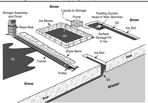
Oil moving both on the surface of ice and underneath it can be concentrated in slots cut in the ice and recovered by skimming with rope mops or other types of skimmers. If the oil in the slot is thick enough, it can be removed using weir skimmers or direct suction.
