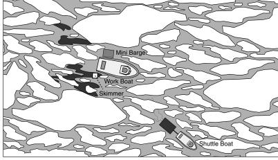
A tug-pushed tank barge, OSRB, OSRV or workboat utilizing various skimmers navigates the spill area collecting oil in pockets of broken sea ice. Onboard cranes place the skimmers into the deepest pools of oil. During collection/recovery, vessels maintain no forward speed and are not using boom.
