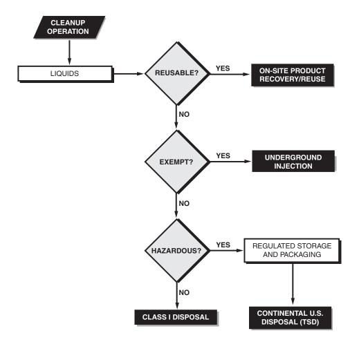
Liquids from cleanup operations include liquid oil; mixtures of oil, water, snow, ice, and/or gravel; used engine oils and hydraulic fluids; contaminated fuels; bilge/ballast waters; stormwater runoff from waste storage areas; and washwaters from decontamination operations.
