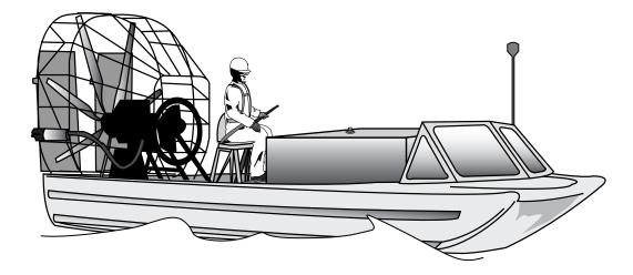
A 300-gallon DOT tank is mounted on a freighter airboat. Liquid is pumped from a recovery site pit, trench, or tank with a 2-inch trash pump onboard. The boat hauls the liquids to a disposal, transfer or storage site.
