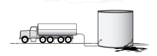
Typically, transfer from a tank would be required if a stationary storage tank either was damaged or developed a serious integrity problem, or if a vacuum truck rolled over on the road and was damaged. Tank holes can be patched by different methods including plug and dike, wooden stakes, and patch kits.
