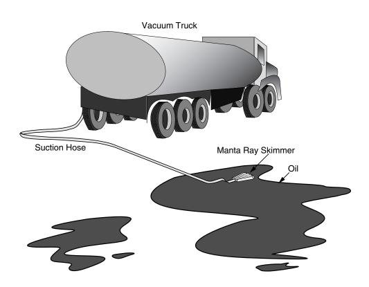
For spills off pad or road, a vacuum truck can effectively reach out 200 feet. If the oil is pooled on water, a Manta Ray skimmer head is attached to the hose extending from the vacuum truck. The hose or skimmer head is placed in the pooled oil for recovery. SRT staff man the hose or skimmer head and move it to other pooled areas as necessary. A Super Sucker can also be used for direct suction.
