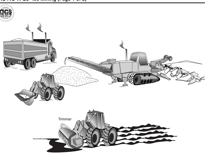
During the winter, ice rubble piles can form at shorelines and manmade structures in the Beaufort Sea. Oil entrained in these piles can be accessed by removing the oiled ice with an ice-miner that grinds up the ice and deposits it in a pile that can be picked up with a front end loader and hauled away by dump truck.
