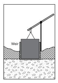
The Fairchild gate weir provides a closable opening for an existing storage trench or deadarm along a river bank. Oil moving on the river is deflected so that it enters the recovery weir into the storage area, and the liquid flow can be controlled as necessary.
