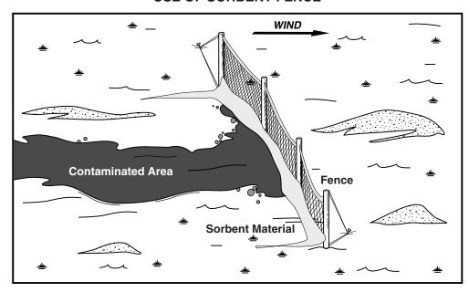
Sorbent pads and rolls can be used onshore to remove small pools of liquid or oil layers on rocks or man-made structures. If the spill is at the shoreline, sorbent boom can be deployed and backed up with conventional containment boom as necessary to keep the oil from drifting away.
