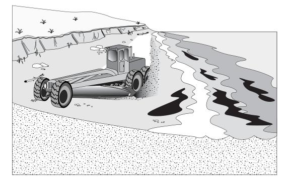
Sediment reworking/surf washing accelerate natural degradation by exposing oil and oiled materials to higher levels of physical (wave) energy.
