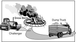
Oil can be burned on any solid surface provided the oil is thick enough to support combustion. This includes tundra, ice, snow, or gravel.
