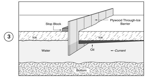
Various techniques that are used on land can also be used on solid ice. (1) Partial trenches or through-ice slots can be dug in the ice surface with a trencher to encourage oil flow to a collection point. (2) The skirt of a containment boom can be set in a shallow trench to provide additional containment. (3) Another approach is to insert a plywood or metal barrier in a slot so that the barrier freezes in place. This tactic can be used to divert under-ice oil to a recovery point.
