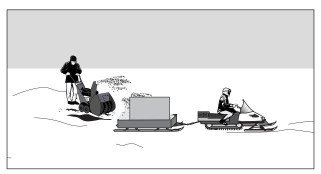
Lightly misted snow can be cleaned up using a snow blower and snow machine with trailer. The snow can be cleaned up either directly off of the ground or by using brooms to sweep oiled snow into windrows for more effective recovery. Once the trailer is full, it is transferred by snow machine to a front-end loader on the gravel pad or road. The loader then transfers the snow into dump trucks on the pad or road.
