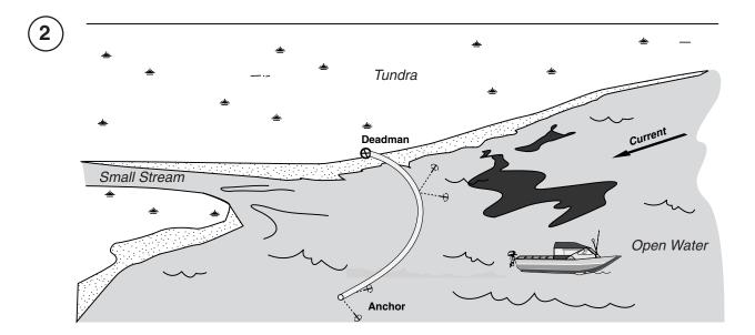
Boom is placed across small inlets and creek mouths identified as sensitive areas. Exclusion booming is used where currents are less than 3/4 knot and breaking waves are less than 0.5 foot in height. The boom is either (1) anchored from shore to shore across the mouths of streams or (2) at an angle to a shoreline to guide oil past the sensitive area. Crews with work boats deploy and tend boom along the shoreline in marshes and inlets.
