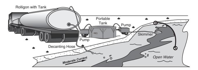
A Rolligon pulls the empty 10,000-gallon trailer tank to a storage site. Liquids are pumped from a temporary tank into the trailer tank using a 4-inch trash pump. The Rolligon then pulls the trailer cross-country and transfers the liquid to a waiting vacuum truck or temporary storage tank on a pad or road. The Rolligon works under ACS's permit for emergency tundra travel.
