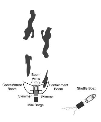
Deployable arms off both sides of the skimming vessel are configured with containment boom and skimmer. The skimmer vessel can advance at a maximum speed of 3 knots, giving an increased encounter rate and maneuverability in recovery operations.
