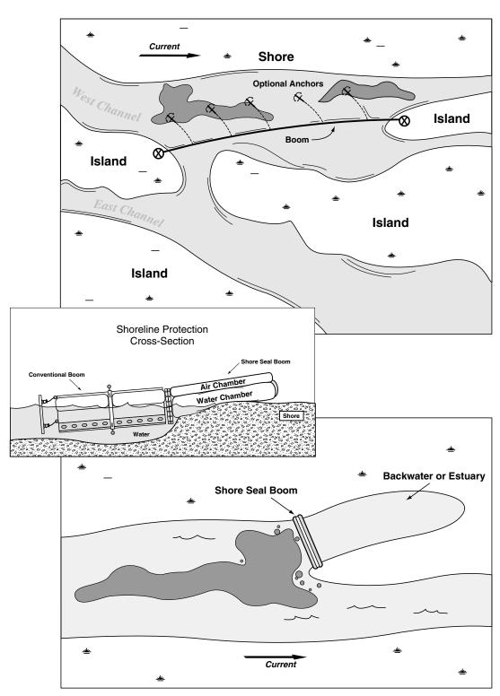
Either conventional boom or a Shore Seal boom can be used to exclude oil from a sensitive area. For example, the Shore Seal boom can be used in shallow water to boom off a backwater, or a conventional boom can be placed across the mouth of a side channel to keep oil out. In addition, Shore Seal boom can be connected to conventional boom to protect the shoreline.
