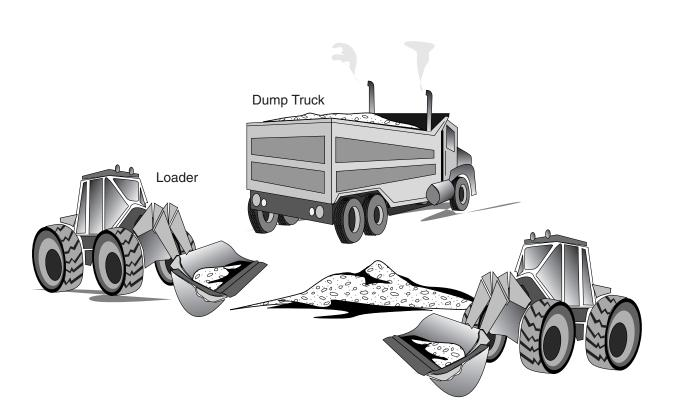
Oiled gravel not considered a regulated waste is excavated with a front-end loader into dump trucks, which then drive to a temporary storage site or a disposal site. Contaminated gravel is stockpiled in temporary lined and diked containment areas.
