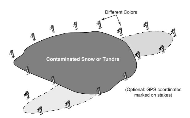
The extent of an oil spill on snow or tundra is delineated so that the oil can be found if subsequent snowfall or windblown snow covers the spill.
