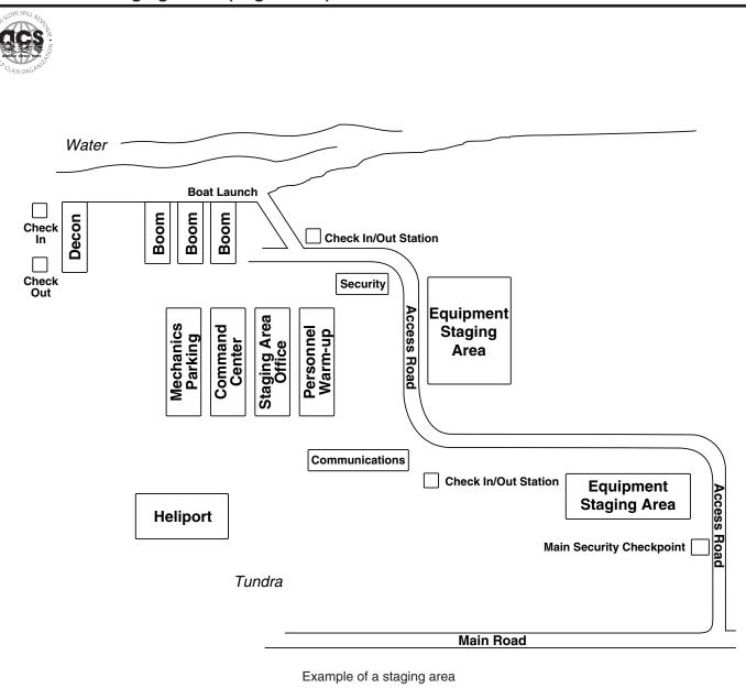
A staging area is a location where personnel and equipment are temporarily placed for tactical deployment during an oil spill response. The staging area provides a system for receiving, tracking and documenting all personnel, equipment, and supplies coming into and out of the staging area from North Slope and out-of-region locations.
