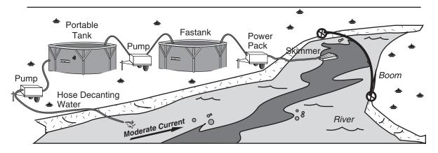
When oil is being skimmed from the water surface, it is likely that considerable volumes of water will be recovered as well. Decanting excess water from oily water storage is an important tool to reduce the volume of oil water that must be taken for disposal.
