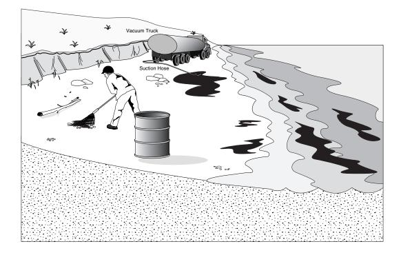
This group of physical methods involves removal of the oil or oiled materials (sediments, debris, vegetation etc.) from the shore zone to a location where it can be disposed of.
