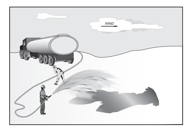
An area of lightly oiled snow can be stabilized for recovery by spraying a light water mist onto the contaminated snow to coat it with a thin layer of ice.
