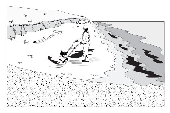
Mechanical tilling/aeration exposes or breaks up surface and/or subsurface oil to accelerate evaporation and other natural degradation processes.
