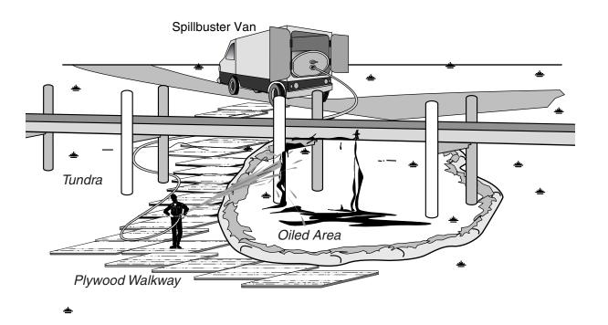
Hot-water, high-pressure washing removes oil from concrete, rock, and metal surfaces. Sorbents, containment boom, and Shore Seal boom prevent re-oiling of adjacent areas. Sorbent boom and skimmers recover oil from adjacent water, while trenches collect surface and subsurface oil.
