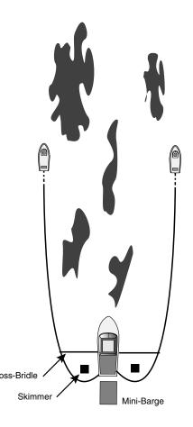
NOTE: This operation may also be conducted using a work boat with integrated oil recovery system and built-in recovered oil storage tank. This option is ideal for handling smaller spills, as well as supporiing larger responses.
