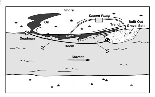
A natural or man-made deadarm trench can be used along the bank of a river to keep oil from migrating downstream from a spill on land. The deadarm will serve as a control point downstream of where the oil is entering the river. Deflection boom is deployed to help divert the oil into the deadarm, which may be lined with an impermeable liner.
