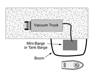
Work boats tow recovered oil-laden mini-barges or floating storage bladders to a waiting OSR platform (tank barge, OSRV, or tanker vessel). Towing speed is 5 knots. The mini-barge or floating storage bladder is tied off using appropriate fendering. Before offloading mini-barges, a bonding cable is connected for protection against accidental ignition. A tankerman assists with the entire off-loading operation, and a Declaration of Inspection form will be completed prior to commencing transfer.
