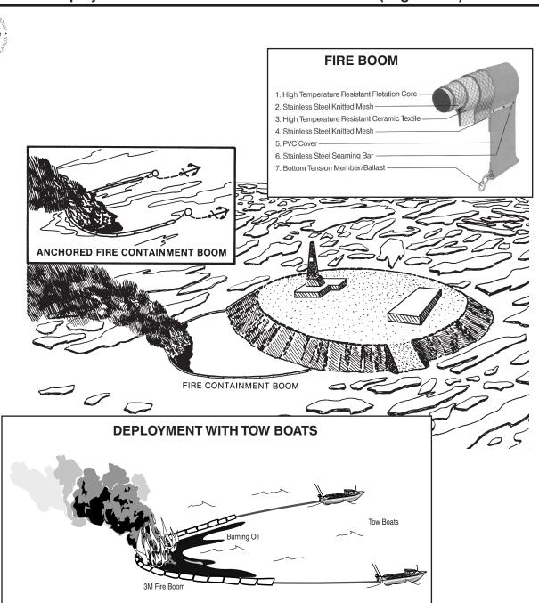
Fire containment boom can be deployed in a stationary mode either anchored to a shore or on the water. In addition, it can be towed like a standard containment boom in a U-configuration to collect oil on water and concentrate it for burning within the boom.
