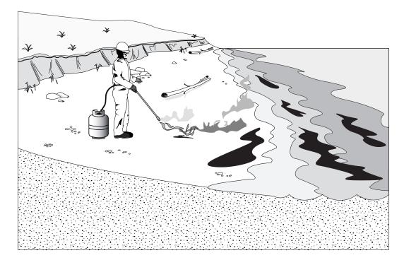
Oil on a beach will not sustain combustion by itself unless it is pooled or has been concentrated in sumps, trenches, or other types of containers. This technique is used primarily where combustible materials, such as logs or debris, have been oiled and can be collected and burned, or where vegetation, such as a marsh, has been heavily oiled.
