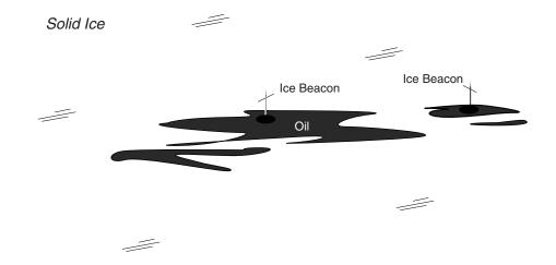
Helicopter operators deploy ice beacons into the slick. The beacon system consists of a GPS receiver, antenna, and beacon equipped with a transmitter. Beacon positions are transmitted to the Command Center via e-mail.
