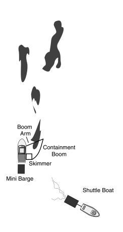
A skimmer vessel (tug-pushed tank barge, OSRB, OSRV or workboat) deployes a skimmer off one side in a boomarm configuration. The skimmer vessel can advance at a maximum speed of 3 knots, giving an increased encounter rate and maneuverability in recovery operations.
