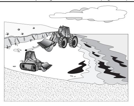
Mechanical removal is more rapid than manual removal but generates larger quantities of waste. The method of operation varies considerably depending on the type of equipment that may be available and on the ability of that equipment to operate on a section of shore. The cleaning efficiency for each type of equipment is expressed in terms of the rate of cleaning that can be achieved and the amounts of waste that are generated.
