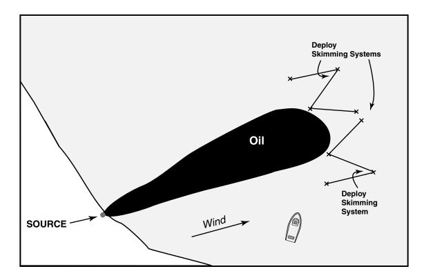
Lengths of deflection boom are anchored in a "W" configuration. Boom sections up to 1,000 feet long are oriented at an angle to the wind and to each other. Oil encountering the center "V" of the boom becomes more concentrated at the downwind end of the configuration and is recovered with a positioned skimming system. Oil is collected from the pockets of the "V"s with a vessel with a skimmer and mini-barge.
