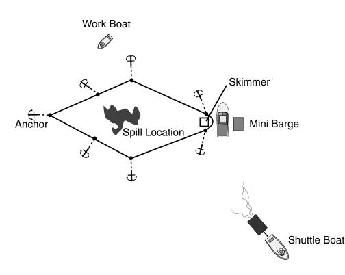
During a subsea pipeline break a diamond-patterned boom can be deployed around the break. A skimmer can be used at any point of the diamond to ensure collection regardless of the wind direction.
