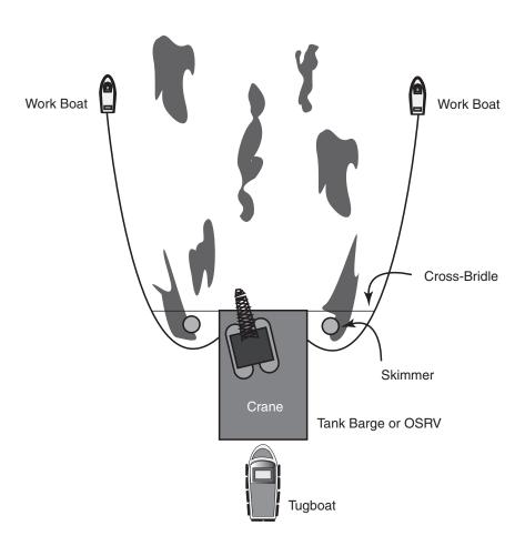
Two work boats each tow 1,000 feet of ocean boom into a J-shape to make a 700-foot sweep. The boom is inflated and deployed from the deck of the tank barge or OSRV. A crane lifts a skimmer from one side of barge's deck into the apex of the boom. The crane positions the skimmers where the oil is deepest. The barge pumps up to 80% of its free water back into the boomed area. The task force advances at a speed no greater than 0.7 knot.
