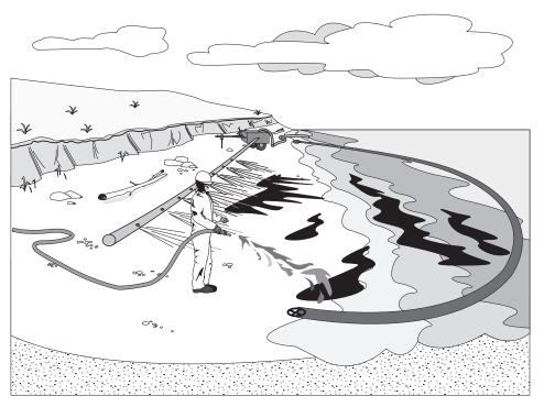
Physical removal involves a variety of washing or flushing tactics to move oil from the shore zone to a location for collection and removal. The variables that distinguish each tactic are pressure and temperature. For all these tactics, booms or other methods of trapping and containment are used to collect the oil for removal.
