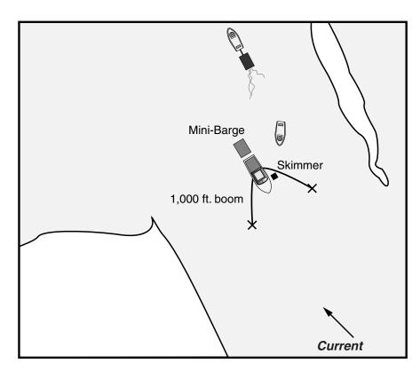
A V-shaped boom configuration is anchored with two booms of 1,000 feet each, with a typical sweep opening of 800 feet. Anchors are placed as appropriate. A skimmer will be tied in at the apex. A workboat supports the skimmer and tends the boom. The skimmer pumps oil and water into a mini-barge anchored immediately downcurrent.
