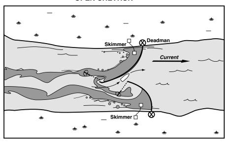
Chevron boom configurations are also for use in fast water. Two booms are deployed from an anchor in the middle of the stream and attached to each bank. A chevron configuration is used to break a slick for diversion to two or more collection areas. An open chevron can be used where boat traffic must be able to pass. (The two booms are anchored separately midstream, with one anchor point upstream or downstream of the other).
