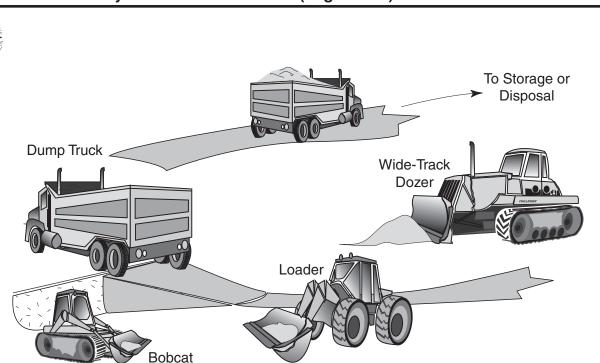
Snow provides a good sorbent material for oil and forms a mulch-like mixture that is easily removed with heavy equipment such as front-end loaders and dump trucks. A Bobcat replaces the front-end loader in hard-to-reach or tight quarters.
