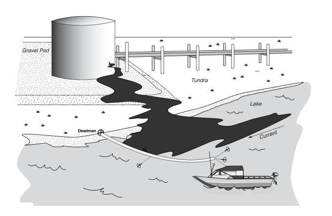
During breakup and summer, lengths of conventional boom can be deployed on a lake or flooded tundra once there is enough open water available. The boom deployment techniques are the same as those in open water.
