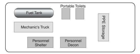
A barge can be used for support operations during a spill. Such operations include the following:
