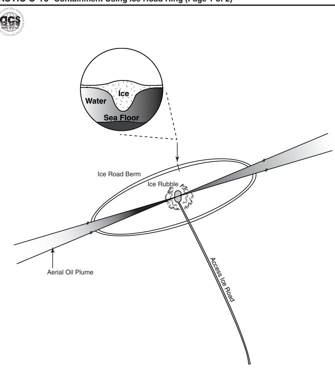
For a blowout that is depositing oil on top of solid sea ice, an ice road can be constructed around the source at a safe distance. Since the ice road causes the sea ice to deflect downward under the road, an under-ice barrier is created to the movement of any oil that may have gotten under the ice. The road also serves as a surface barrier because it is higher than the surrounding ice, and will provide a working platform into the breakup season, when the ice inside the ring decays.
