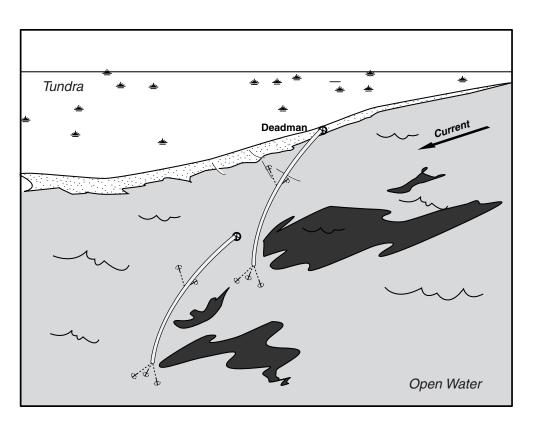
Deflection booming is often used where the water current is greater than 1 knot or where exclusion boom does not protect the shoreline. Deflection booming diverts oil to locations that are less sensitive or more suitable for recovery.
