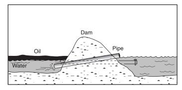
An underflow dam can be used when there is too much water flow to allow for a complete blockage of a drainage channel. The dam is built of earth, gravel, or other barriers such as sandbags or plywood sheets. A MegaSecure dam may also be used if water depth is shallow enough.
