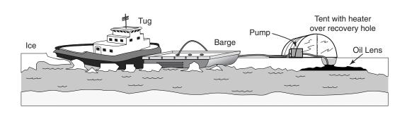
Oil trapped under solid ice or in a lens within solid ice can be removed by augering into the oil lens and pumping out the oil. If the ice is thick enough to support heavy equipment, the oil can be pumped directly into bladders or other portable tanks and hauled to shore. In the case of thin nearshore ice, the oil can be pumped to storage containers on shore. Finally, if the site can be reached by an ice-strengthened tug-and-barge combination, the oil can be pumped directly into the barge.
