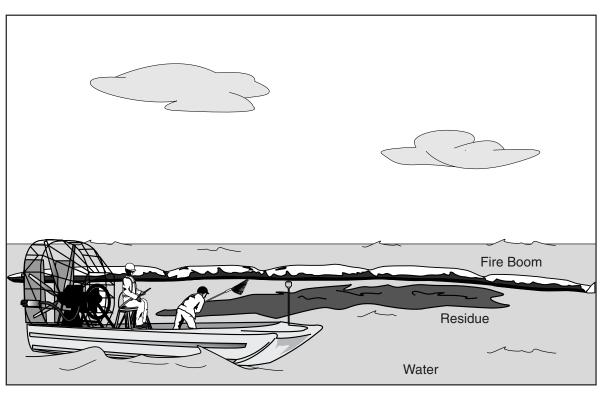
The type and amount of residue from an in-situ burn of oil on water depend on the starting oil type and condition, as well as the way in which the oil is contained and/or herded throughout the burn. If wind or currents are available to push burning oil against a barrier (boom, ice, steel structure, etc.), adequate combustion thicknesses will be maintained for a much more efficient burn. The residue may be an inch or more thick.
