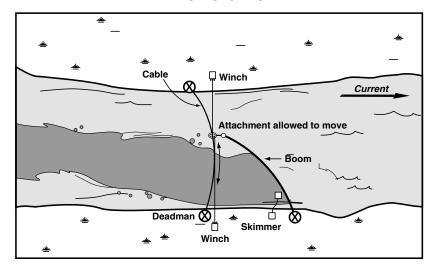
Catenary (currents less than 1/4 knot): The boom is attached to an anchor on one bank, and the other end is towed to the other bank and attached to an anchor there. The current naturally puts the boom in a "U" shape ("catenary"). The deployment and maintenance of a single long boom can be difficult and labor-intensive. It is usually used for recovery operations.
