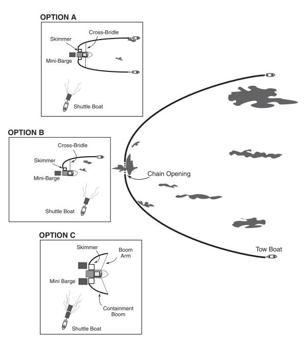
The length of boom and boom swath width are determined by the towing capacity of the boats and the water depth. For a swath width of 650 feet, two work boats each pull 1,000 feet of ocean boom. (Shorter lengths of boom may be necessary to avoid boom planing or entrainment based on sea conditions).
