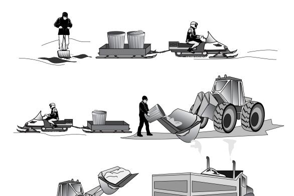
Broom and shovel the oiled snow into piles. The piles are then transferred with shovels to garbage cans, totes, or similar containers. Once a container is full, it is transferred with a snow machine or Argo to a front-end loader near the gravel pad or road. The loader then transfers the snow into dump trucks on the pad or road.
