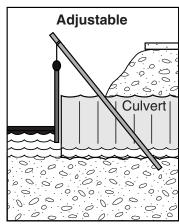
A culvert is blocked using sheet metal, plywood barriers, or inflatable culvert plugs. Use a full block only when the culvert will be blocked for the entire cleanup operation, if the oil floating on the water will not contaminate additional soil or tundra, and if blocking the water flow will not threaten the road. Otherwise, an adjustable weir should be used.
