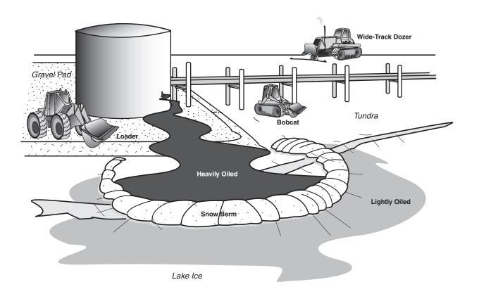
A snow berm is built around the areas of heaviest oiling to contain oil or diesel spilled to tundra and/or ice in winter. A rubber tracked, wide-track dozer drives around the spill with its blade angled towards the spill, pushing snow into a berm. Once the perimeter has been covered with an initial berm, the dozer shores up areas, as necessary.
