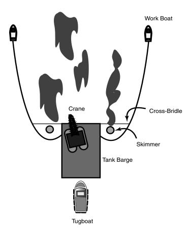
Two work boats each tow 400 feet of ocean boom from the barge into a J-shape to make a 300-foot sweep. Length of boom depends on the ice conditions. A crane lifts a skimmer from one side of the storage barge's deck into the apex of the boom. The crane positions the skimmers where the oil is deepest, and the barge fills with recovered liquids.
