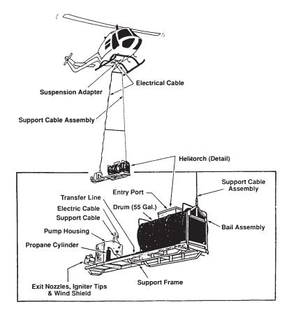
Numerous methods are available for the ignition of floating oil. Hand-held pyrotechnic devices such as ACS's Dome igniters can be armed and tossed by hand from a helicopter or vessel. If such devices are unavailable, one can often make a simple though effective igniter on location using oil-soaked rags, sorbents, or even a roll of toilet paper. When it is unsafe to use such igniters, and particularly when a large, intense ignition area is needed, a Heli-torch may be used.
