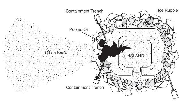
Trenching can help recover oil from a blowout on an offshore island in winter when the sea ice is solid.
