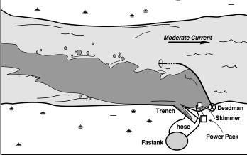
Portable skimmers are easily mobilized, transported, and deployed and can be used in most spill situations for recovery. They can be used to recover oil from containment areas such as the apex of a diversion boom or natural or artificial deadarms. The typical portable skimming system includes:
